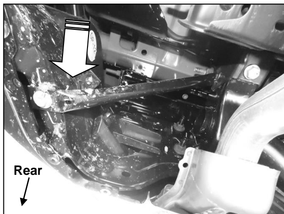
(Fig 5) Remove the bolts attaching the outer bumper supports to the bottom of the bumper (arrow)
