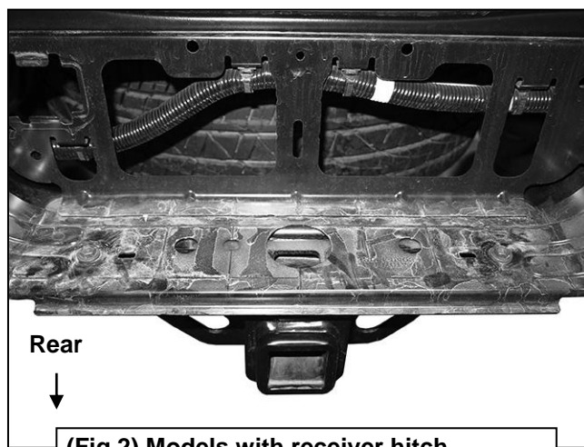
(Fig 2) Models with receiver hitch, remove plastic cover from top of bumper
