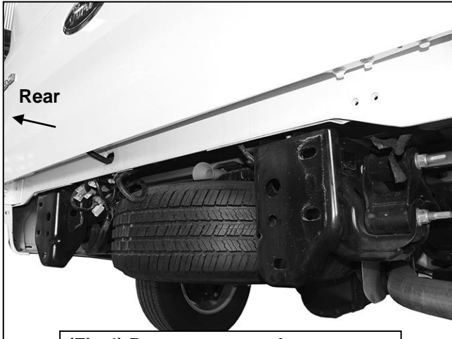
(Fig 4) Bumper removed, passenger side pictured without receiver hitch
