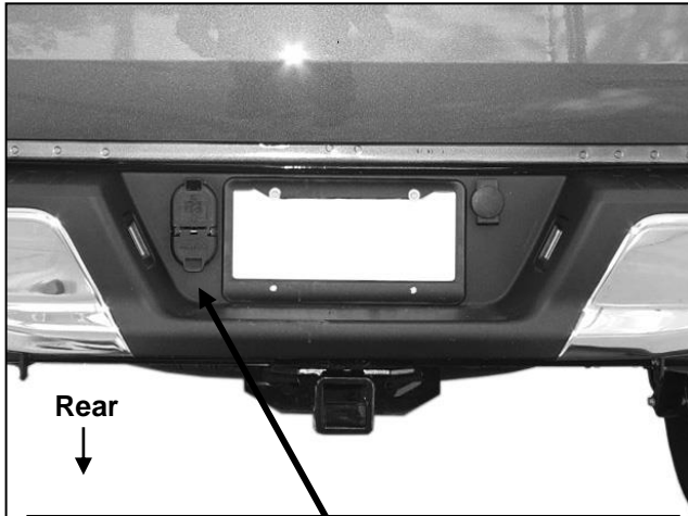
(Fig 1) Unplug and remove 7-wire trailer plug
