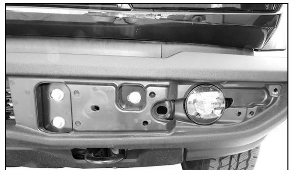
(Fig 2) Models with plastic bumper cover (see Fig 1), remove bumper pads from bumper (driver/left side pictured)
