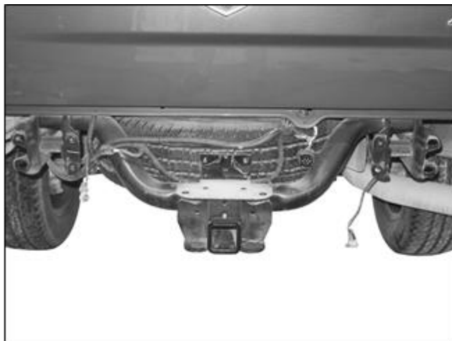
(Fig 8) Example of factory bumper brackets with (4) mounting holes per side, only outer mounting holes will be used
