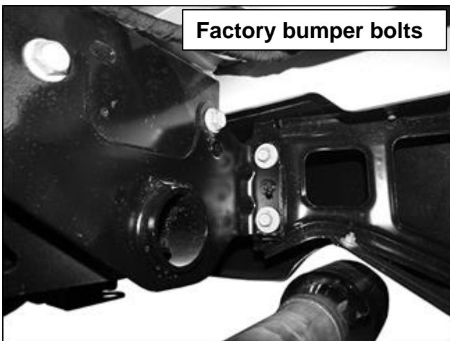
(Fig 5) Example of factory bumper bracket with (2) hex bolts pictured from behind bumper
