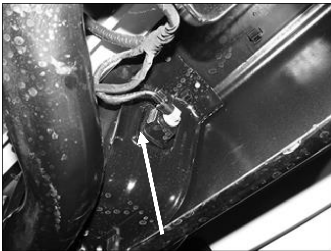
(Fig 3) Unplug license plate lights and all wiring harnesses leading to the bumper
