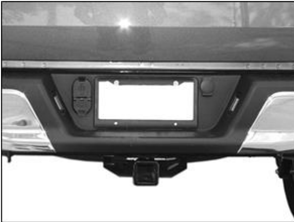
(Fig 1) Unplug and remove 7-wire trailer plug
