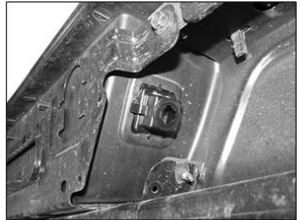
(Fig 2) Unplug license plate lights
