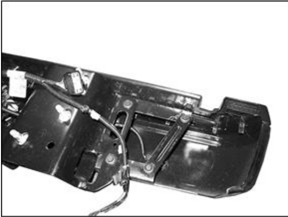
(Fig 5) Disassemble factory bumper to remove lights, plugs, sensors and harness
