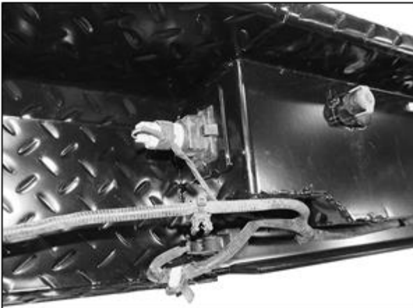
(Fig 9) Install lights, sensors, trailer plug and harness before installing Bumper
