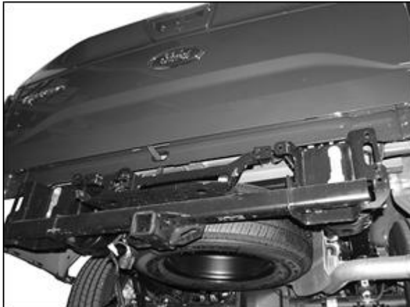
(Fig 17) Reinstall integrated receiver hitch/bracket assembly on models with "HD Towing" package
