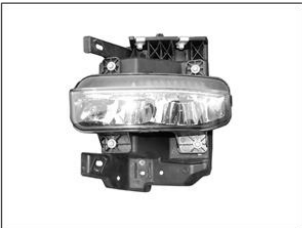
(Fig 20) Remove the (4) bolts to remove the driver/left LED fog light from outer plastic housing if equipped
