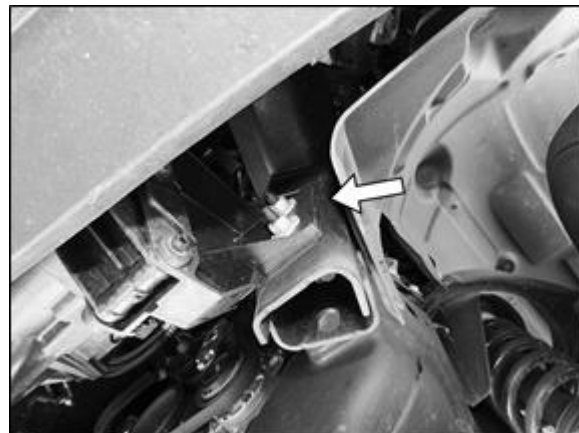
(Fig 2) Models with automatic air dam, unplug and remove air dam, (Driver/left side pictured from below - arrow)
