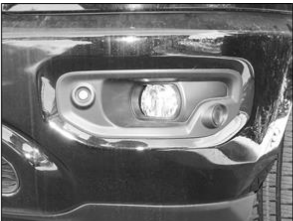
(Fig 22) Remove driver/left round fog light from housing if equipped
