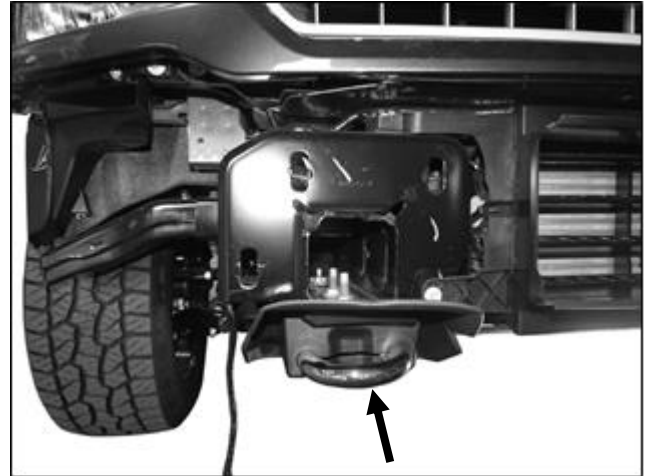
(Fig 4) Remove the tow hooks and plastic covers, if equipped
