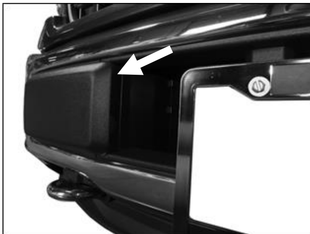
(Fig 1) From behind bumper, release metal clips attaching plastic bumper pad to the bumper
