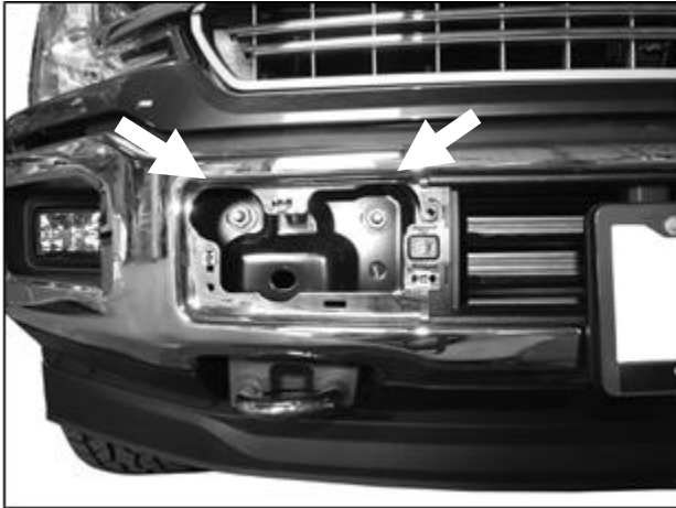
(Fig 3) Remove (2) factory hex nuts from each side
