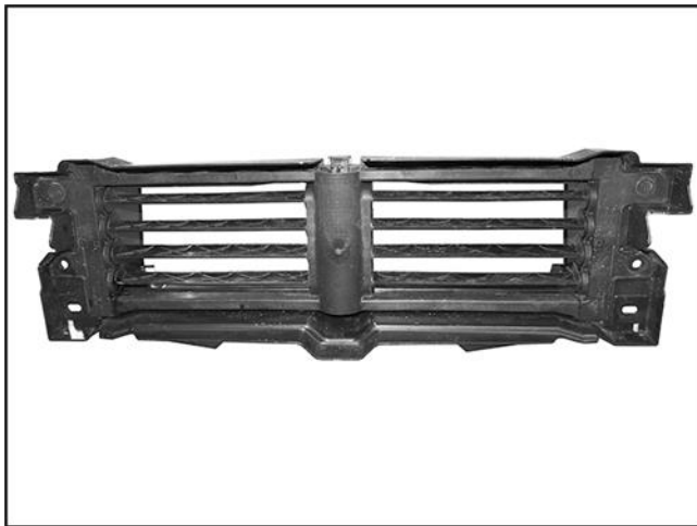
(Fig 15) Remove inner shutter assembly from plastic outer housing (if equipped)
