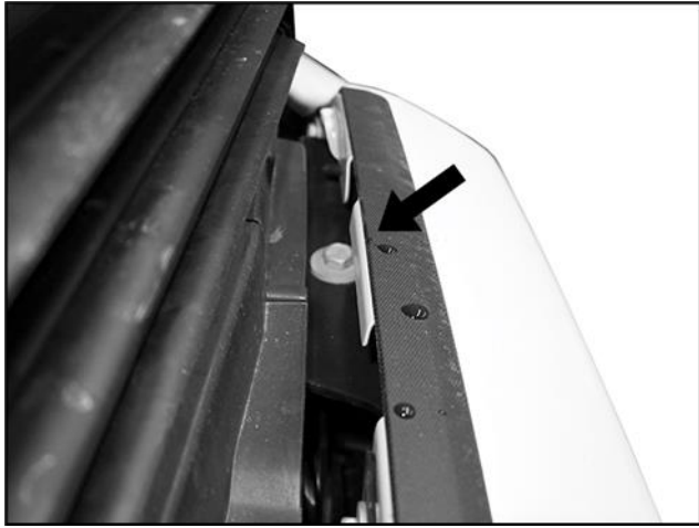
(Fig 9) From above, remove the hex bolts attaching the bumper assembly to the frame bumper brackets (top visible-arrow)
