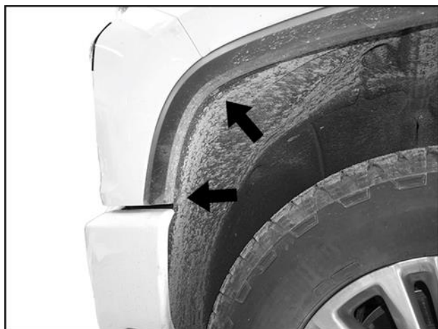
(Fig 1) Release hardware attaching fender liner from plastic panel (fascia-see arrows)
