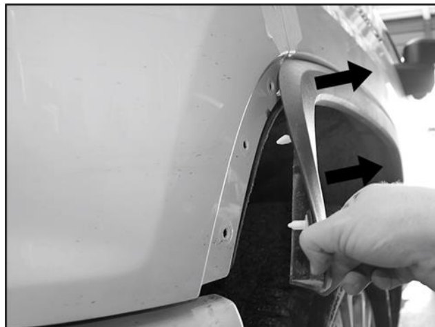
(Fig 2) Pull front end of fender flare out and away from fender. Do not remove flare, only release the front section
