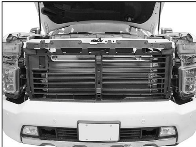
(Fig 7) Grille and fascia removed
