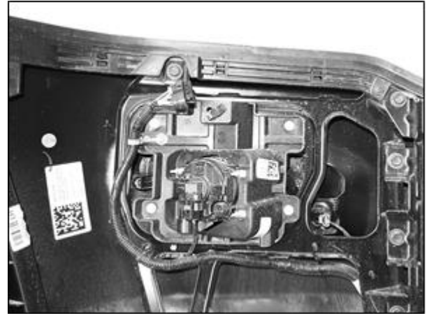
(Fig 14) Models with round fog lights, remove light assembly from outer plastic housing. Passenger / right side pictured
