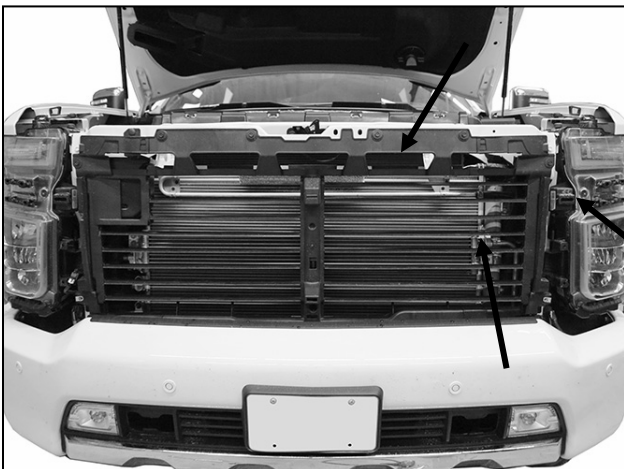
(Fig 7) Grille and fascia removed
