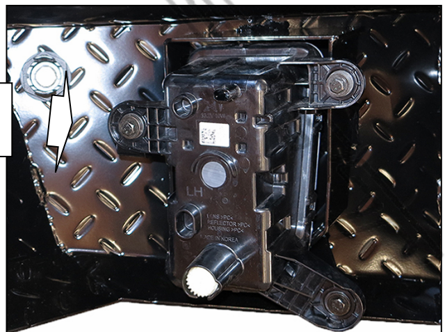
(Fig 28) Attach fog light to mounting tabs on driver/left side of Bumper
