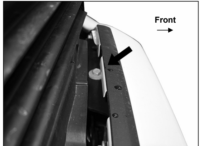
(Fig 10) From above, remove the hex bolts attaching the bumper assembly to the frame bumper brackets (top visible-arrow)
