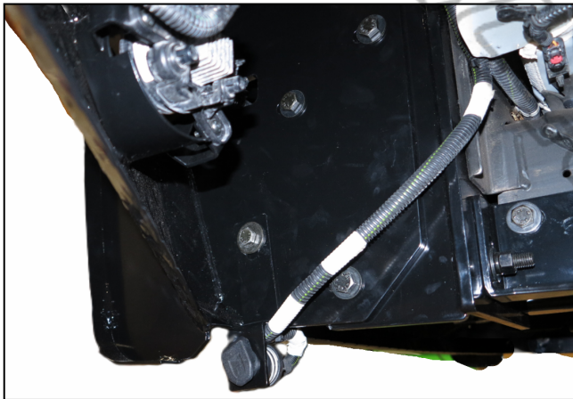
(Fig 28) Driver/left side of Bumper installed (Optional Block Heater installed)
